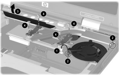
Removing the Heat Sink Screws
